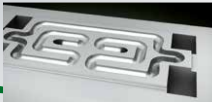
Mold with cooling channels
