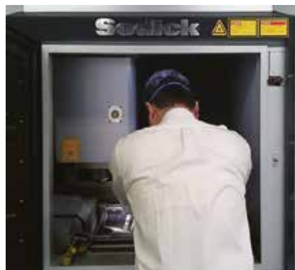
Wide-open operation door
