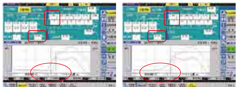
Injection setting screen and velocity pressure waveform without PDT control
